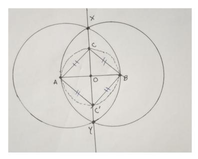
Step (i) Let AB = amiles. Take a compass and Make A as certer and B as Radius and Drow circle T1. step(ii) Aake another circle T2 by considering Bas center and A as radius. step(iii) Circle T, intersect circle T, at Two point X, & Y. step[iv] pass a line through XY which intersect AB at Oby using storightedge step(v) make a circle T3 whose center is 0 and radius is 0A. 900 step(vi) Circle T3 cut the XY at two point c' and C'. Hence : - Path ACB and AC'B becomes two possible ways.
